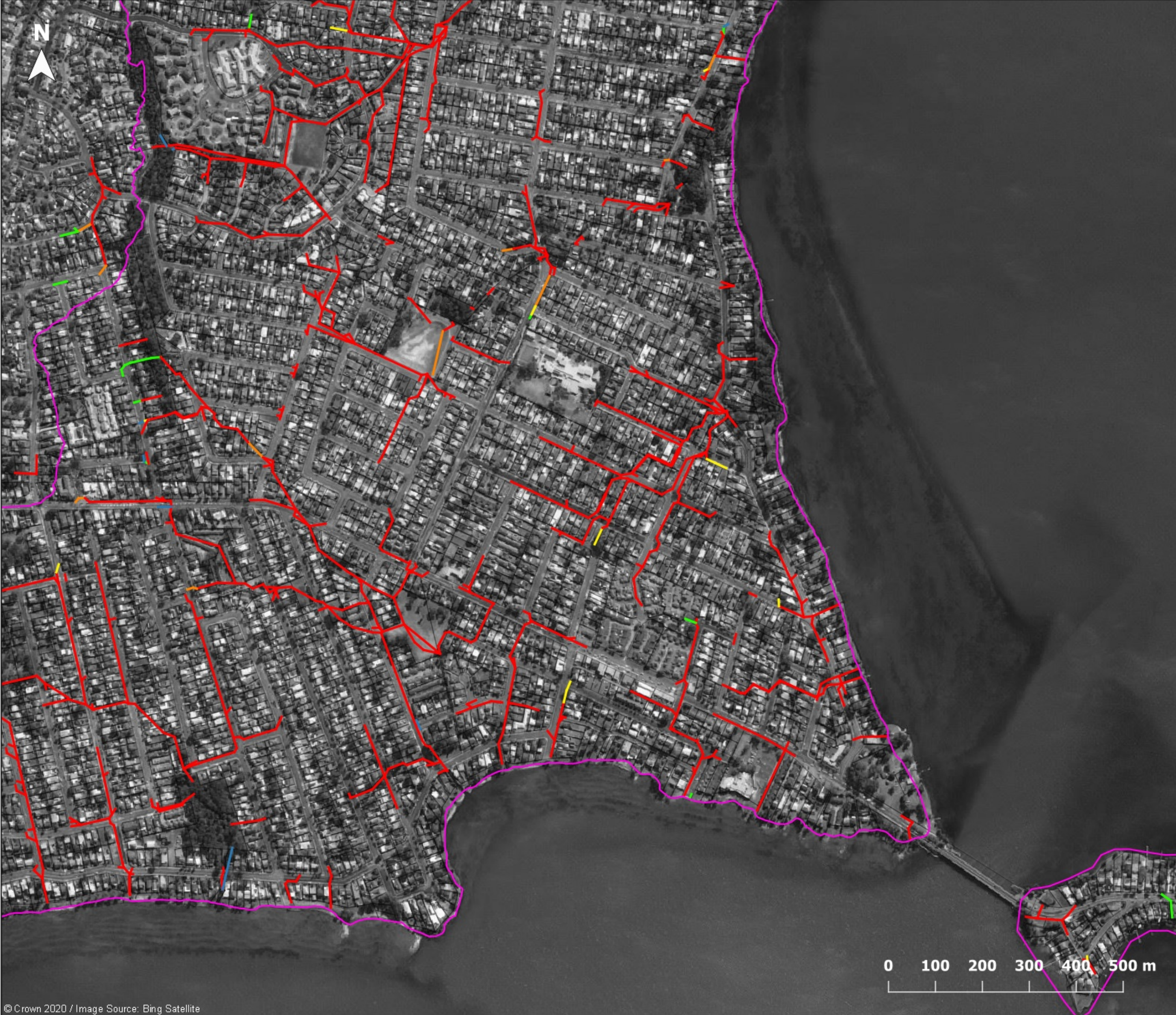
Figure J4.5 Probable Maximum Flood Pipe capacity
