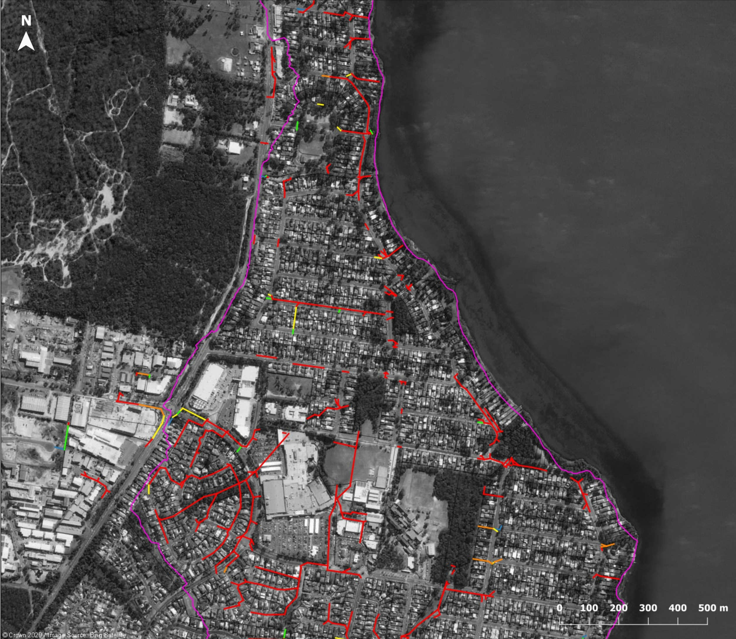
Figure J4.6 Probable Maximum Flood Pipe capacity
