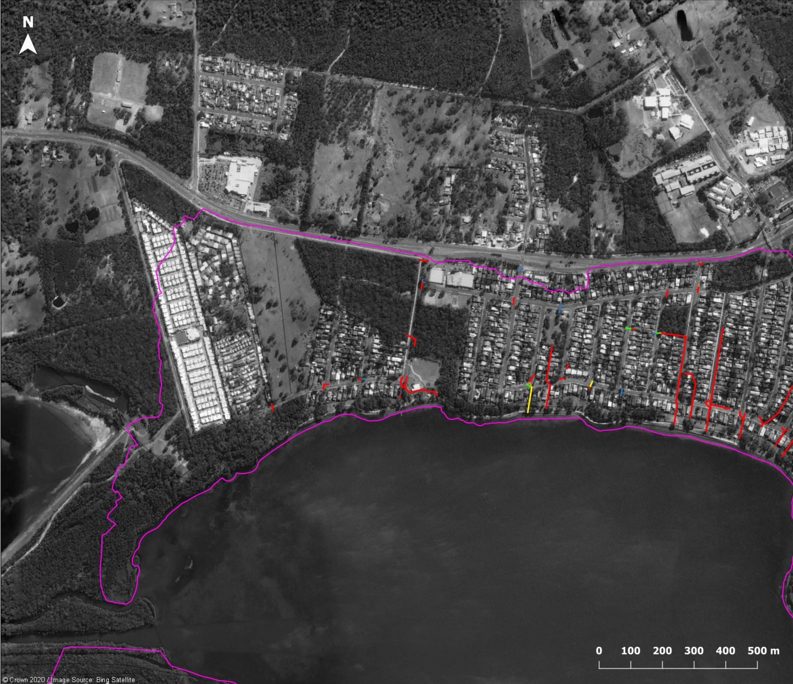
Figure J4.12 Probable Maximum Flood Pipe capacity
