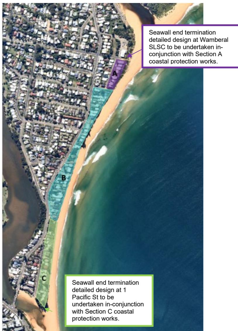
**Figure 4.1: Divisions for staged seawall construction**
